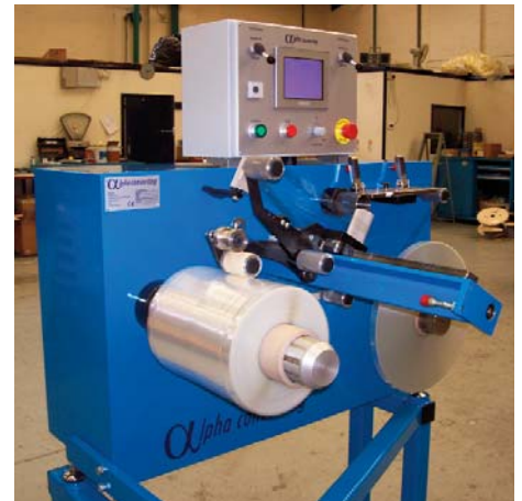
ALPHASPOOL RSM – here being used to wind a narrow tape of film from a pancake reel to a traverse wound spool.
